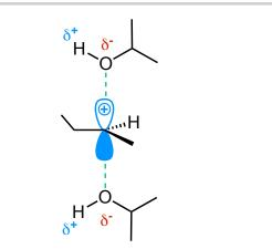
To stabilize the cation (empty p-orbital in this case), the solvent will orient itself such that the negative end of the O-H bond dipole will be closer to the positively charged carbon. 4. Shown below is a stepwise mechanism for the hydration of an alkene.
